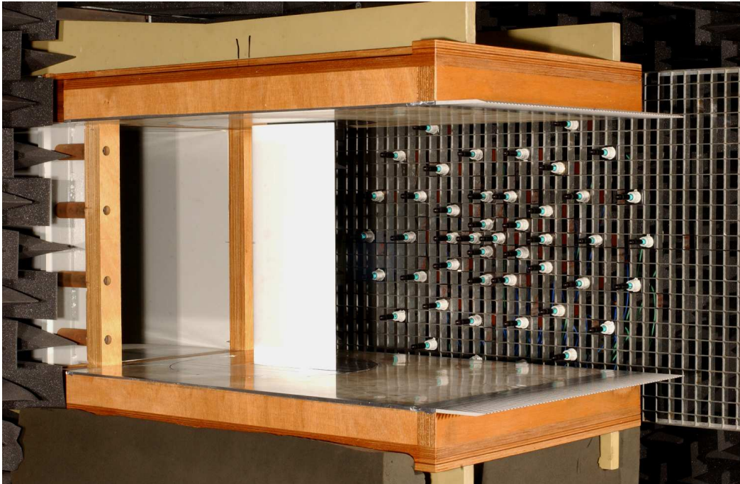
Figure 7-3: NLR anechoic wind tunnel set up with acoustically lined endplates and microphone array.
