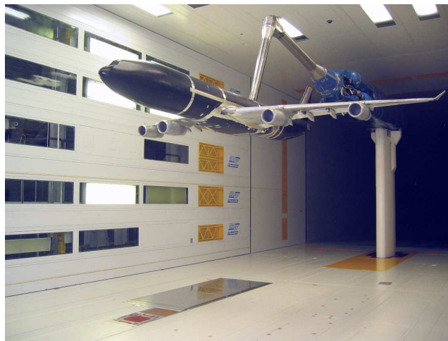
Figure 4-2: Test set-up in DNW closed test section, with wall arrays on the tunnel floor.
