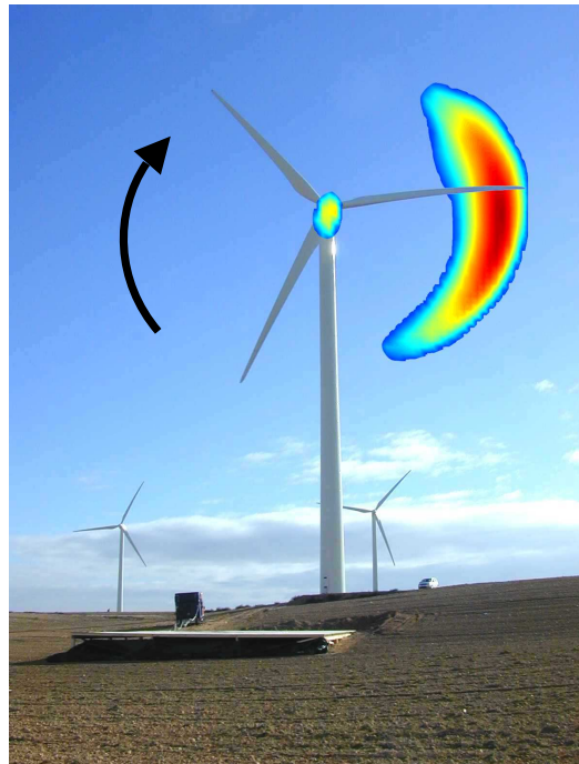
Figure 5-1: Test set-up with G58 wind turbine and microphone array platform. The noise sources in the rotor plane (averaged over several rotations) are projected on the picture.
